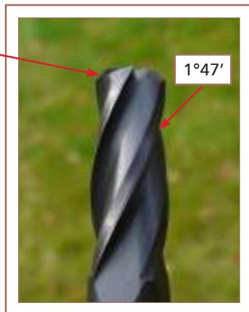
Premilling of conical holes result in longer tool life of thread mill
